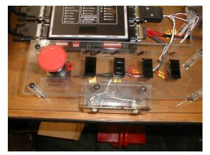
are the wearable heads-up display outputs that are a part of our driver's station and the feedback steering control on the robot. This steering control is described in more mechanical detail on its own page, but electronically below. We also spent a lot of time developing software and programming for many different inputs, including potentiometers, a yaw rate sensor and Banner optical sensors.
