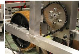
wheel diameter, in conjunction with the 12.75:1 gear ratio in the gearboxes and a 1:1 ratio from the gearbox to the wheels,
