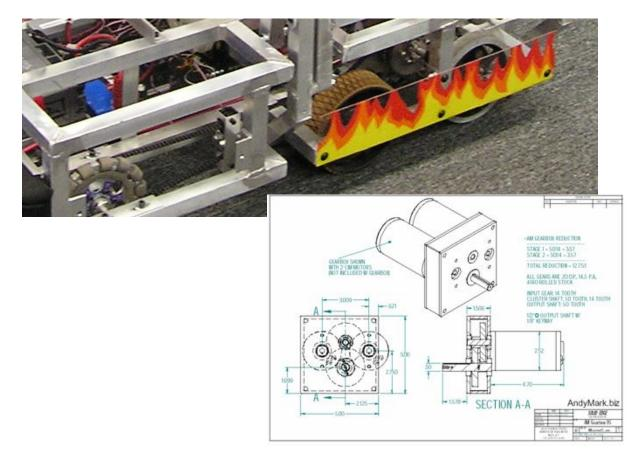
The traction wheels have been placed on each side, close to the middle of the robot, to enable the HOTBOT to achieve a near "zero point" turning radius. Each main traction wheel is powered by a CIM motor attached to an Andy Mark gearbox. By choosing a 6-inch
