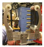
The end-effector allows the HOTBOT to pick up tubes in any orientation and place them in any position on the rack. The end effector is mounted on a hinged joint to meet the initial packaging constraints. The end effector is forced into its game configuration by a 60 lb gas spring. A 50 lb gas dampener is also used to smoothly change configurations at the start of the match. This joint allows the arm some flexibility during game play to resist damage if the arm is
