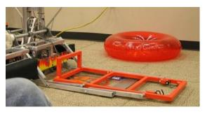
The HOTBOT lift system was engineered with two four-bar linkages on each side of the robot. The lift system was designed to package as thin as possible. We assumed when the lifts were designed that the majority of robots have at least 1 inch of ground clearance. If another robot has this clearance, they should have no trouble entering onto our lift system. We felt that a four-bar linkage lift system was the most efficient way to elevate a robot 12 inches from
