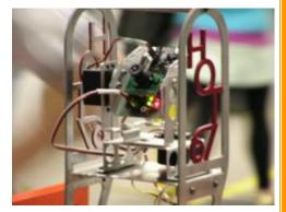
light is to the right or the left of the center pixel default, the robot corrects itself to point towards the light. This is also controlled by a proportional algorithm so that the closer you get, the less the robot turns to try to correct itself. Once it gets to a certain tilt position, the robot stops driving, lowers the arm, and powers out the tube.
