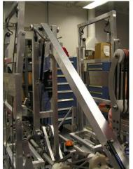
was mounted on the arm to aid the motor when the arm is rotated up. A chain tensioner was engineered into the arm drive system to counteract high strain on the motor, motor mounts, and arm brackets. The chain tensioner absorbs the forces produced when the arm is
